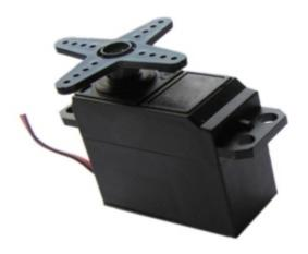
Similar to the way you used pulses to PWM on LED in the Colour Mixing Lamp Project, servo motors expect a number of pulses that tell them what angle to move to. The pulses always come at the same time intervals, but the width varies between 1000 and 2000 microseconds. While it's possible to write code to generate these pulses, the Arduino software comes with a
